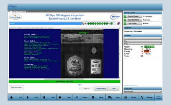
The control software WeSysExec controls the complete vision system and acts as user interface for configuring the vision application.
